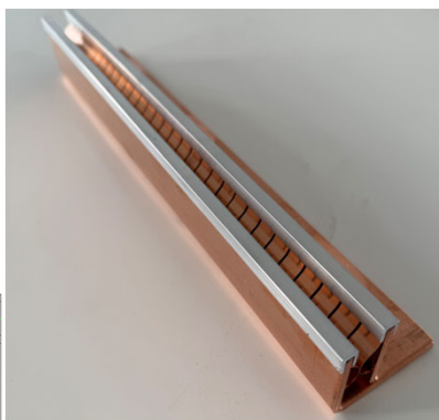
CISPR test table fast ground connection part Made by copper panel and beryllium copper finger
