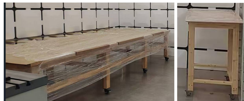
Non-Metal Test table Made by wooden without metal screw
